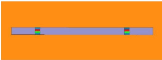
Fig 3.2 PIN Diodes in the slot.
